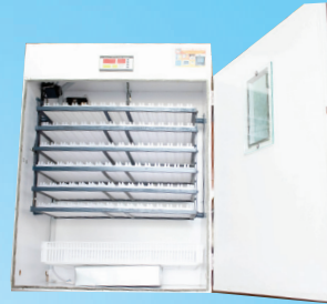
NH-176/200 Capacity:176/200eggs Size:730*580*950mm Weight:43kg
